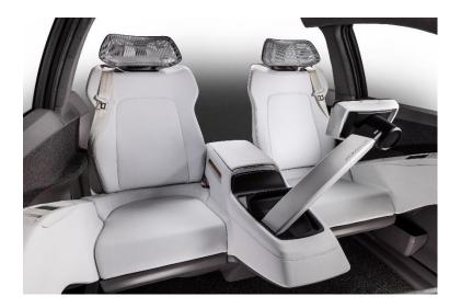
**EVI 3:** Through the development of EVI and the Smart Cabin Seat, Yanfeng's experts challenged themselves to simplify the vehicle interior while keeping the functionality that users expect. The Yanfeng solution builds them back in a unique way, in an all new module that incorporates both front seats, integrated floor console, steer-by-wire input system, HMI, displays, seatbelts and airbags, in addition to a HVAC microclimate system for thermal comfort.
