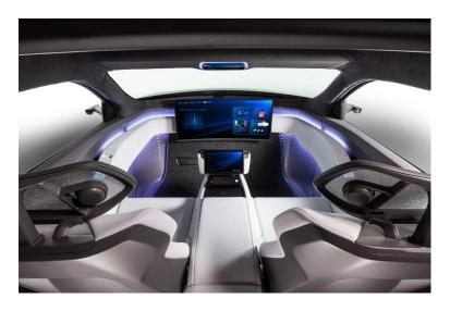
**EVI 1:** At the 2024 CES, Yanfeng debuted its EVI (Electric Vehicle Interior) concept, a vision for future vehicle architecture, that eliminates the traditional instrument panel, and incorporates all key features and interior functions into a Smart Cabin seat, including an active headrest with integrated audio, safety systems, smart surfaces, and storage and charging integrated into the seat.
